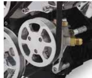
▲ Pump for Remote Tank
