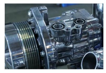
2. With the plate removed, you will see the two sealing o-rings. Leave these on the compressor and be careful not to damage them.
