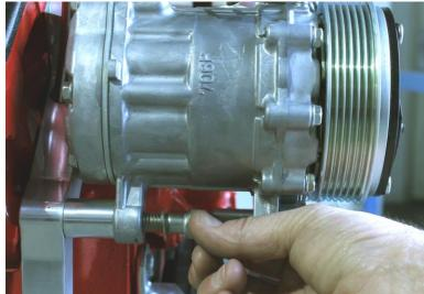
3. Use 1) 7/16-14 X 2-1/4" socket cap screw, 1) 7/16 washer and 1) 1" spacer to fasten the compressor to the rear bracket. Use anti-seize on the threads but do not fully tighten at this point.
