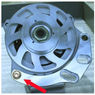
1. Use 1) 8MM-1.25 30MM button head bolt to attach the alternator adjusting bracket to the alternator. Use anti-seize but don't tighten yet.
