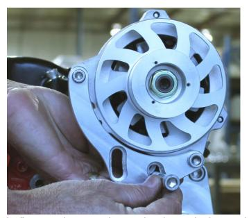
2. Use 2) 2" spacers between the rear bracket and adjusting bracket, apply anti-seize and fasten with 2) 3/8-16 X 2-3/4" socket caps screws. Do not tighten yet.
