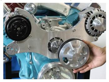
1. Install the water pump pulley using four 5/16-18 X 5/8" socket cap screws. Apply Loctite to the threads and tighten fully while using caution to prevent over torqueing.
