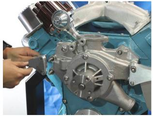
1. Install the air compressor bracket over the 3/8" studs protruding from the water pump housing.
