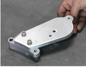
1. Attach the small rear power steering bracket to the large front bracket using two  $5/16 \times 1''$  socket head cap screws and washers. Make sure the recess for the 3/8'' mounting bolt on the large front bracket is facing forward ("down" in this picture), away from the block.
