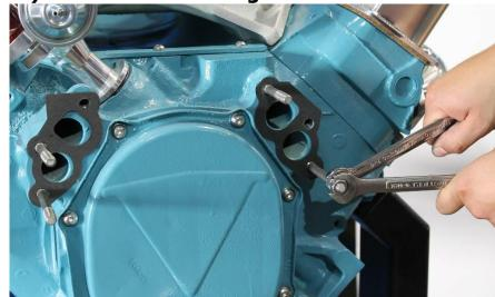
1. Apply RTV silicone sealer to the ends of the four mounting studs and thread them into the holes in the block surrounding the two water pump water passages as show here. Use the following studs:
