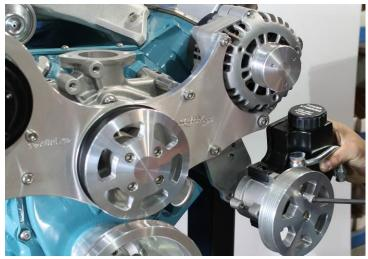
1. If you purchased the kit with a power steering pump with an attached reservoir, install the hard line on the pump. Hand tighten the fitting only as you will be removing it later, after
