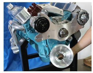
1. Install the crank pulley using six  $5/16-18 \times 1-1/2''$  socket cap screws and lock washers. Apply Loctite to the threads and tighten fully while using caution to prevent over torqueing.
