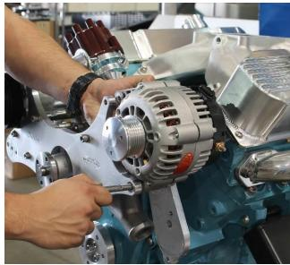
1. Install the alternator to the main plate using the 10MM-1.5 X 80MM socket head cap screw through the main plate and bottom mounting hole of the alternator.
