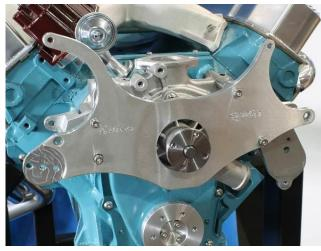
1. Install the main bracket to the stainless steel stand-off posts using four M8 X 1.25 X 25mm socket cap screws and AN washers. Use antiseize on the threads. Do not fully tighten the fasteners at this time.
