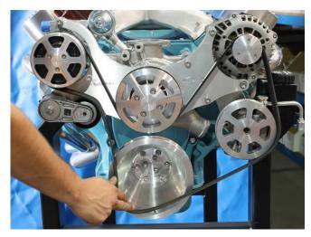
2. Route the belt onto the pulleys as shown.
