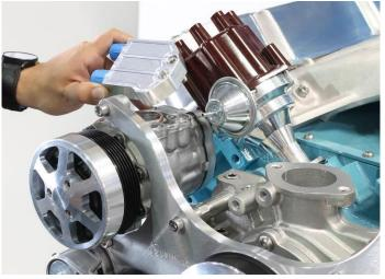
3. Using caution so as not to damage the o-rings, install the compressor manifold to the compressor using two M8 x 25mm
