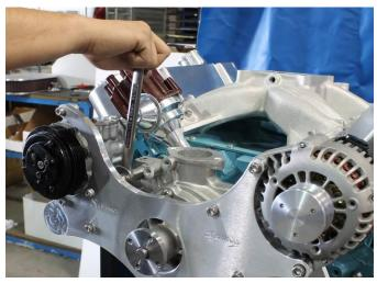
1. With all of the components attached to the main plate, fully tighten the stainless steel stand-off posts and all of the fasteners attaching components. Use caution to prevent over torqueing.
