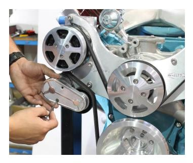
4. Install the aluminum tensioner cover using two  $10-32 \times 3/4"$  socket head flat head screws. Tighten fully while using caution to prevent over torqueing.
