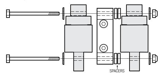
When using MS109-11 Coil Mount Kit with Brackets, install the coils onto the coil mounts using 1/4-20 X 2 1/4" bolts and aluminum spacers as shown.
