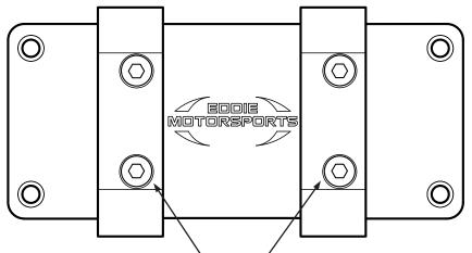
When using MS109-11 Coil Mount Kit with Brackets, install the coil mounts onto the mounting plate, with the left mount bolt hole offset facing "in" and the right mount bolt hole offset facing "out" as shown.
