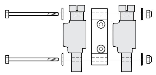
Install the coils onto the coil mounts using %-20 X 2 %" bolts as shown.
