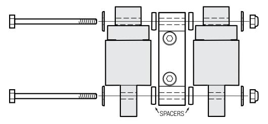
When using MS109-10 Coil Mount Kit only **WITHOUT** Brackets, install the coils onto the coil mounts using  $\frac{1}{2}$ -20 X 2  $\frac{3}{4}$ " bolts and aluminum spacers as shown.
