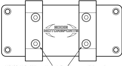
When using MS109-11 Coil Mount Kit with Brackets, install the coil mounts onto the mounting plate with the bolt hole offset facing "in"/towards each other as shown
