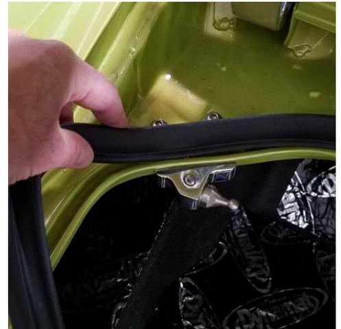
5.) Reinstall the weather stripping back into the weather strip channel.
