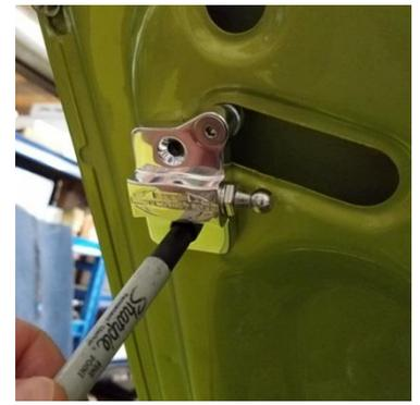
2.) "Hook" the "L" bracket into the top pocket in the deck lid. Slide the bracket until it contacts the inside edge of the top corner of the pocket and the bracket is parallel to the outer edge of the seam on the deck lid (Image A). Once in position, mark the two holes for drilling.
