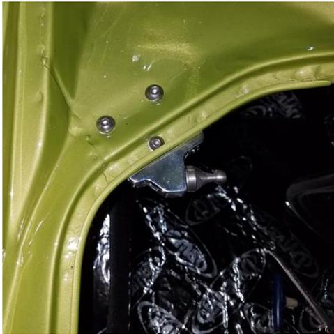
4.) From the underside of the drip rail, use the lower strut mount as a template and drill the additional two 5/16" mounting holes. Apply anti-seize to the 5/16" X 3/4" button head bolt and fasten the bracket permanently.
