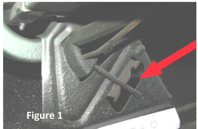
**NOTE: Once the spring tension is released, if you do not plan on saving the bars, you can cut them with a die grinder to ease removal.**
