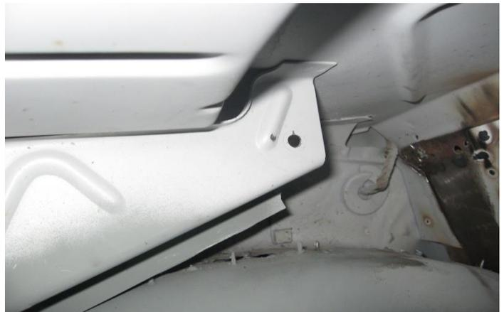
5. With the struts facing the center of the car, slide the hinge into the pocket strut first. Push ball stud through the 5/16" hole, and secure with a washer and nut. Install the new hinge pins and bend the tab back down.
