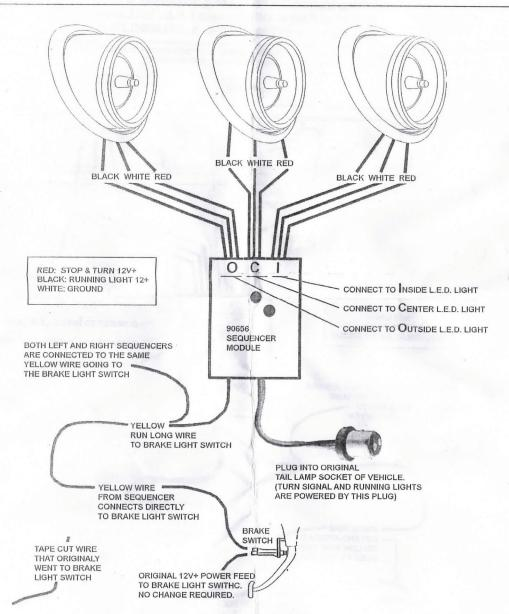
Wiring Instruction For Adding Sequencer Module To United Pacific 1969 Camaro L.E.D. Tail Lamps Part Numbers CTL6901LED-L & CTL6901LED-R
